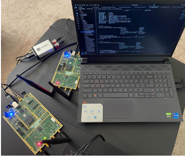
Figure 4: Testbed setup for 5G end-to-end communication. The gNB (USRP: bottom-left) and UE (USRP: top-right) are connected to a laptop and GPSDO.
